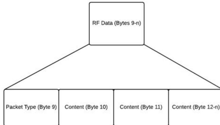
All subsequent packets will be sent in bytes 9-n of the transmission. The number of content bytes will vary depending on the packet type. Packet types are outlined in Section 5.
